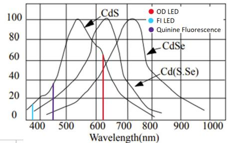
Filter Selection: 400 nm glass long-pass filter is used to block the FI excitation light source
