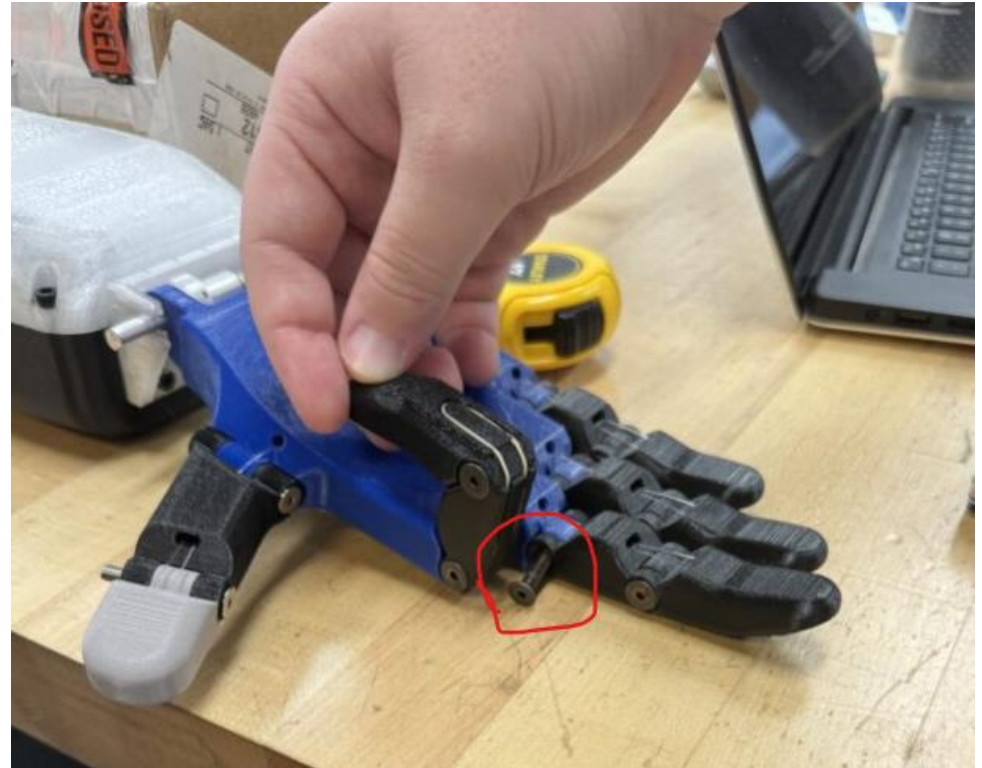
Loosened fastener after 12" test
