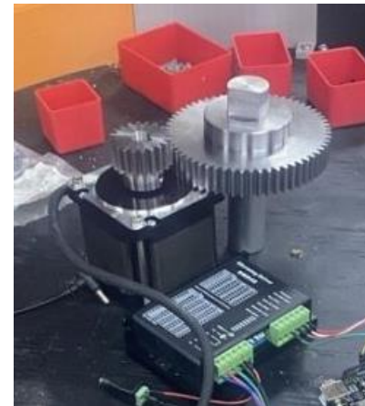
Motor & Gear System providing rotation
