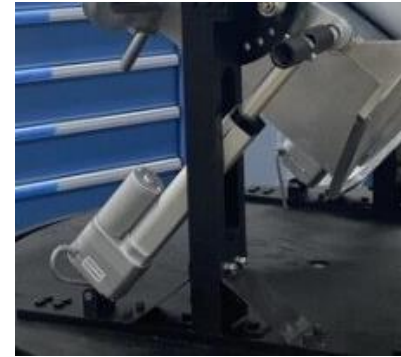
Linear actuator (mounted to support beam) providing tilt
